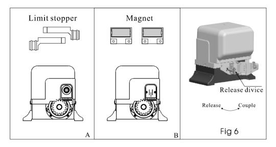
Move the gate manually to the open limit and close limit, mark the points on the Rack, then, fix the limit Stoppers or Magnets at the limit points on the Rack.
