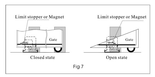
NOTE: Magnet must be 10mm~20mm space from the operator, and must be same height with the Magnetic switch inside of the Operator Blue Magnet is for Open Limit, Red Magnet is for Close Limit.
