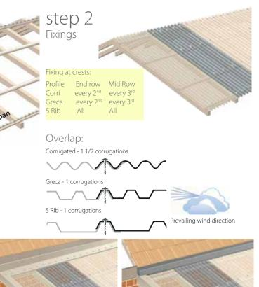
AGAINST A WALL/FASCIA - Fit barge capping to edge of sheet and apron flashing at the wall or fascia. Secure using recommended fixing screws.
