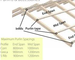
Ensure that your roof pitch is at least 5°, ie. 88mm rise per lineal metre. This will ensure adequate water run off.
