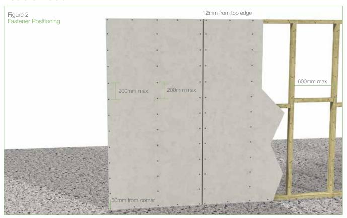
Durascpae $^{\text{TM}}$  panels should be installed vertically with all sheet edges fully supported. The centre joints must coincide with the
