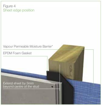
Position the underlap sheet on every stud 3mm past the centre of the stud to ensure the fasteners fixed at the edge of the sheet have adequate distance into the stud.
