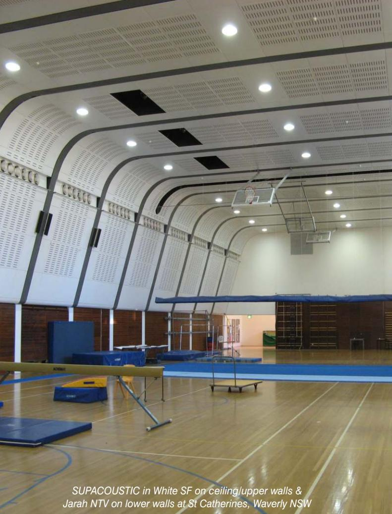
*SUPACOUSTIC in White SF on ceiling/upper walls & Jarah NTV on lower walls at St Catherines, Waverly NSW*
